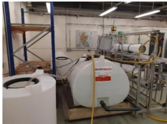
Figure 15 - High-recovery batch RO prototype installed in the UoB laboratory (A and B) front view, (C) side view, (D) Back view.
