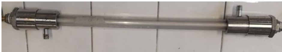
Figure 3 CUT single membrane (8mm) tubular module
