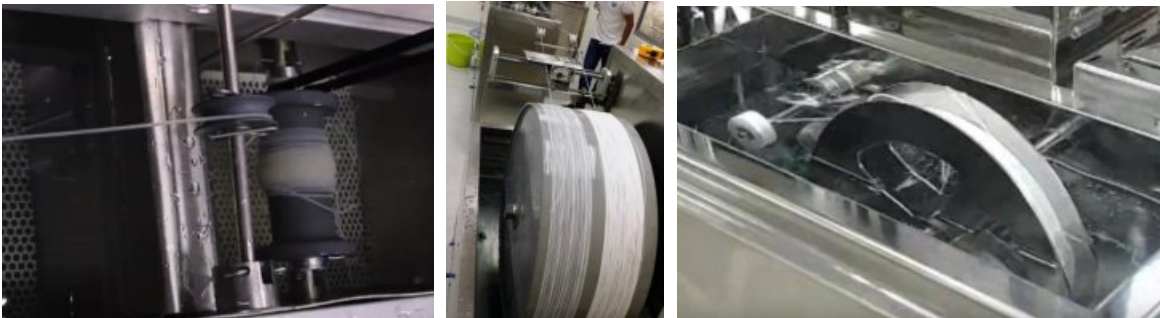
Figure 8 - Examples of spools for winding hollow fibers.
