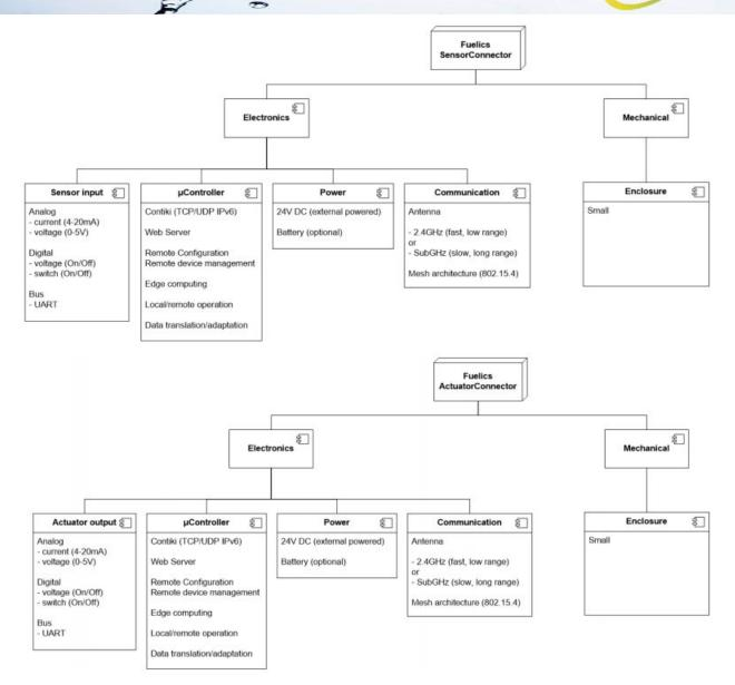
Fuelics R&D has prototyped so far the aggregator using the abovementioned analysis. We do estimate that within 2022 a full production cycle of sensorconnectors, actuatorconnectors and aggregators in the sub GHz and 2,45GHz band will be released and tested in Demokritos lab and then in the industrial demos.
